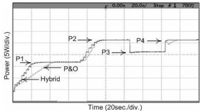
Fig. 14. Comparison of hybrid and P&O algorithm subjected to benchmark loading pattern. Power states  $P_1$ ,  $P_2$ ,  $P_3$ , and  $P_4$  correspond to solar conditions with ideal maximum power of 12.0, 21.92, 16.51, and 21.92 W, respectively.
