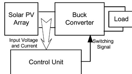
Fig. 1. Block diagram of the MPPT system.
