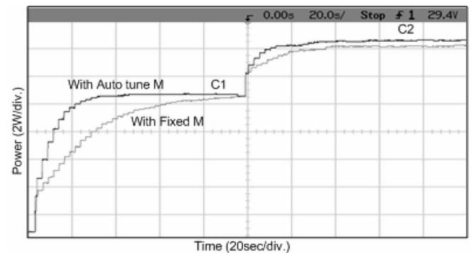
Fig. 9. Startup and steady-state and step change performances of autotuned and manually tuned (for 37.5 W two-panel), i.e., fixed- $M$  variable-step-size algorithms. C1 and C2 are at the insolation levels corresponding to maximum powers of 10.0 and 14.0 W, respectively.
