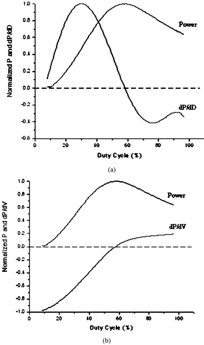
Fig. 4. Approximated and normalized empirical curves. (a)  $P$  and the derivative of  $P$  w.r.t.  $D$ . (b)  $P$  and the derivative of  $P$  w.r.t.  $V$ . These are plotted against the control parameter  $D$ . Curve (a) shows erratic variation of the derivative whereas (b) shows smooth variation. The observations were taken from single PV panel at an insolation level of  $620 \text{ W/m}^2$  at 2.20 P.M. on a clear day in the month of May in New Delhi, India.
